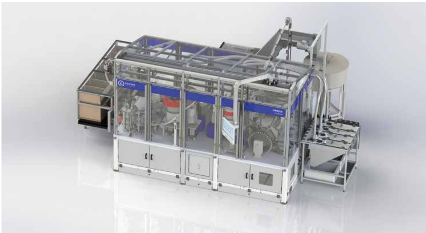
Leonhard Fischer valve assembly cell
